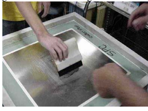
Figure 3: Hand Stenciling of Solder Paste
